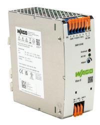
WAGO Eco2 series switching power supply, 24 VDC @ 10A/240W (adjustable), 100-240 VAC nominal input, 1-phase, enclosed, metal housing, 35mm DIN rail mount, cage clamp.
