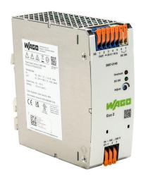
WAGO Eco2 series switching power supply, 24 VDC @ 10A/240W (adjustable), 100-240 VAC nominal input, 1-phase, enclosed, metal housing, 35mm DIN rail mount, cage clamp.
