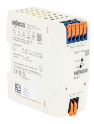
WAGO Eco2 series switching power supply, 24 VDC @ 2.5A/60W (adjustable), 120/240 VAC nominal input, 1-phase, enclosed, plastic housing, 35mm DIN rail mount, cage clamp.
