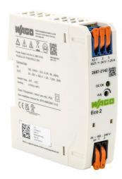
WAGO Eco2 series switching power supply, 24 VDC @ 1.25A/30W (adjustable), 100-240 VAC nominal input, 1-phase, enclosed, plastic housing, 35mm DIN rail mount, cage clamp, NEC Class 2.
