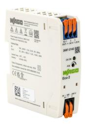
WAGO Eco2 series switching power supply, 24 VDC @ 1.25A/30W (adjustable), 100-240 VAC nominal input, 1-phase, enclosed, plastic housing, 35mm DIN rail mount, cage clamp, NEC Class 2.
