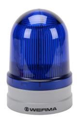
WERMA EvoSIGNAL Maxi TwinLIGHT series LED industrial signal beacon, 120mm, blue, permanent or blinking (1 Hz ON for 480ms), IP66, modular mount, 12/24 VAC/VDC. Requires mounting adapter.
