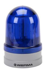
WERMA EvoSIGNAL Maxi TwinLIGHT series LED industrial signal beacon, 120mm, blue, permanent or blinking (1 Hz ON for 480ms), IP66, modular mount, 115-230 VAC. Requires mounting adapter.
