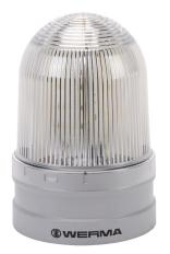
WERMA EvoSIGNAL Maxi Rotating series LED industrial signal beacon, 120mm, clear/white, rotating (180rpm), IP66, modular mount, 12/24 VAC/VDC. Requires mounting adapter.
