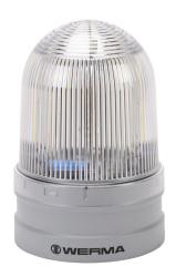
WERMA EvoSIGNAL Maxi TwinFLASH series LED industrial signal beacon, 120mm, clear/white, double flash or EVS (Enhanced Visibility System) flashing (random flashing), IP66, modular mount, 12/24 VAC/VDC. Requires mounting adapter.
