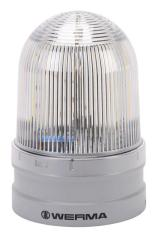
WERMA EvoSIGNAL Maxi TwinLIGHT series LED industrial signal beacon, 120mm, clear/white, permanent or blinking (1 Hz ON for 480ms), IP66, modular mount, 115-230 VAC. Requires mounting adapter.
