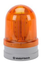
WERMA EvoSIGNAL Maxi Rotating series LED industrial signal beacon, 120mm, yellow, rotating (180rpm), IP66, modular mount, 115-230 VAC. Requires mounting adapter.
