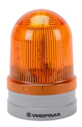
WERMA EvoSIGNAL Maxi TwinLIGHT series LED industrial signal beacon, 120mm, yellow, permanent or blinking (1 Hz ON for 480ms), IP66, modular mount, 115-230 VAC. Requires mounting adapter.
