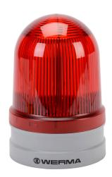
WERMA EvoSIGNAL Maxi TwinFLASH series LED industrial signal beacon, 120mm, red, double flash or EVS (Enhanced Visibility System) flashing (random flashing), IP66, modular mount, 12/24 VAC/VDC. Requires mounting adapter.
