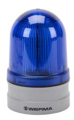
WERMA EvoSIGNAL Midi Rotating series LED industrial signal beacon, 85mm, blue, rotating (180rpm), IP66, modular mount, 115-230 VAC. Requires mounting adapter.
