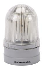
WERMA EvoSIGNAL Midi Rotating series LED industrial signal beacon, 85mm, clear/white, rotating (180 rpm), IP66, modular mount, 115-230 VAC. Requires mounting adapter.
