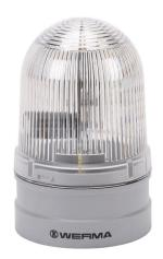
WERMA EvoSIGNAL Midi TwinFLASH series LED industrial signal beacon, 85mm, clear/white, double flash or EVS (Enhanced Visibility System) flashing (random flashing), IP66, modular mount, 12/24 VAC/VDC. Requires mounting adapter.
