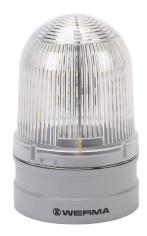
WERMA EvoSIGNAL Midi TwinLIGHT series LED industrial signal beacon, 85mm, clear/white, permanent or blinking (1 Hz ON for 480ms), IP66, modular mount, 12/24 VAC/VDC. Requires mounting adapter.
