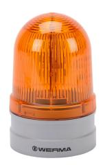
WERMA EvoSIGNAL Midi TwinLIGHT series LED industrial signal beacon, 85mm, yellow, permanent or blinking (1 Hz ON for 480ms), IP66, modular mount, 12/24 VAC/VDC. Requires mounting adapter.
