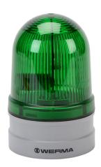
WERMA EvoSIGNAL Midi TwinFLASH series LED industrial signal beacon, 85mm, green, double flash or EVS (Enhanced Visibility System) flashing (random flashing), IP66, modular mount, 12/24 VAC/VDC. Requires mounting adapter.
