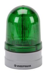
WERMA EvoSIGNAL Midi TwinLIGHT series LED industrial signal beacon, 85mm, green, permanent or blinking (1 Hz ON for 480ms), IP66, modular mount, 12/24 VAC/VDC. Requires mounting adapter.
