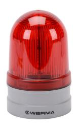
WERMA EvoSIGNAL Midi Rotating series LED industrial signal beacon, 85mm, red, rotating (180rpm), IP66, modular mount, 12/24 VAC/VDC. Requires mounting adapter.
