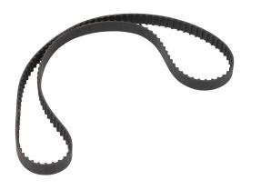
SureMotion timing belt, 1/5in XL pitch, 3/8in wide, 130 tooth, 26in pitch length (circumference), neoprene, fiberglass reinforced.
