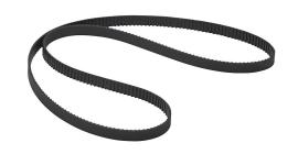
SureMotion timing belt, 0.08in MXL pitch, 1/4in wide, 260 tooth, 20.8in pitch length (circumference), neoprene, fiberglass reinforced. Package of 3.
