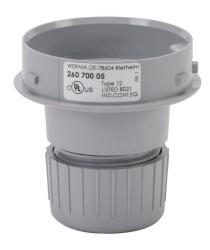
WERMA EvoSIGNAL Mini series tube adapter, tube mount, 1/2in NPT thread type, 62mm diameter, 60mm height, gray, ABS plastic. For use with WERMA EvoSIGNAL Mini industrial signal beacons, audible-visual signal beacons and audible signal horns.
