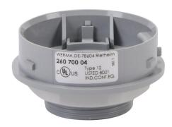
WERMA EvoSIGNAL Mini series PG 29 mounting adapter, panel mount, PG29 thread type, gray, ABS plastic. For use with WERMA EvoSIGNAL Mini industrial signal beacons, audible-visual signal beacons and audible signal horns.
