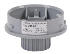
WERMA EvoSIGNAL Mini series mounting adapter, panel mount, M22 x 1.5mm thread type, 62mm diameter, 33mm height, gray, ABS plastic. For use with WERMA EvoSIGNAL Mini industrial signal beacons, audible-visual signal beacons and audible signal horns.
