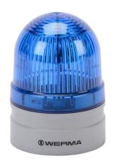
WERMA EvoSIGNAL Mini TwinLIGHT series LED industrial signal beacon, 62mm, blue, permanent or blinking (1 Hz ON for 410ms), IP66, modular mount, 12 VAC/VDC. Requires mounting adapter.
