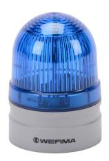
WERMA EvoSIGNAL Mini TwinLIGHT series LED industrial signal beacon, 62mm, blue, permanent or blinking (1 Hz ON for 420ms), IP66, modular mount, 115-230 VAC. Requires mounting adapter.
