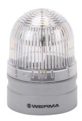
WERMA EvoSIGNAL Mini TwinLIGHT series LED industrial signal beacon, 62mm, clear/white, permanent or blinking (1 Hz ON for 470ms), IP66, modular mount, 24 VAC/VDC. Requires mounting adapter.
