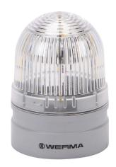
WERMA EvoSIGNAL Mini TwinLIGHT series LED industrial signal beacon, 62mm, clear/white, permanent or blinking (1 Hz ON for 470ms), IP66, modular mount, 24 VAC/VDC. Requires mounting adapter.
