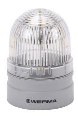
WERMA EvoSIGNAL Mini TwinLIGHT series LED industrial signal beacon, 62mm, clear/white, permanent or blinking (1 Hz ON for 410ms), IP66, modular mount, 12 VAC/VDC. Requires mounting adapter.
