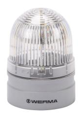
WERMA EvoSIGNAL Mini TwinLIGHT series LED industrial signal beacon, 62mm, clear/white, permanent or blinking (1 Hz ON for 420ms), IP66, modular mount, 115-230 VAC. Requires mounting adapter.
