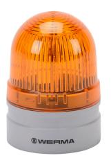
WERMA EvoSIGNAL Mini TwinFLASH series LED industrial signal beacon, 62mm, yellow, double flash or EVS (Enhanced Visibility System) flashing (random flashing), IP66, modular mount, 24 VAC/ VDC. Requires mounting adapter.
