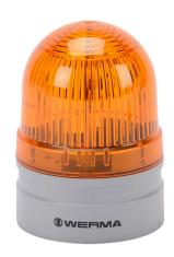
WERMA EvoSIGNAL Mini TwinLIGHT series LED industrial signal beacon, 62mm, yellow, permanent or blinking (1 Hz ON for 410ms), IP66, modular mount, 12 VAC/VDC. Requires mounting adapter.
