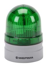
WERMA EvoSIGNAL Mini TwinFLASH series LED industrial signal beacon, 62mm, green, double flash or EVS (Enhanced Visibility System) flashing (random flashing), IP66, modular mount, 12 VAC/VDC. Requires mounting adapter.
