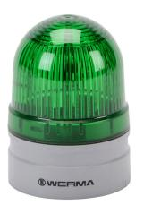
WERMA EvoSIGNAL Mini TwinLIGHT series LED industrial signal beacon, 62mm, green, permanent or blinking (1 Hz ON for 470ms), IP66, modular mount, 24 VAC/VDC. Requires mounting adapter.
