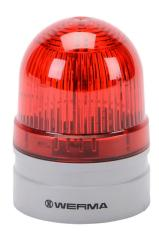
WERMA EvoSIGNAL Mini TwinFLASH series LED industrial signal beacon, 62mm, red, double flash or EVS (Enhanced Visibility System) flashing (random flashing), IP66, modular mount, 24 VAC/VDC. Requires mounting adapter.
