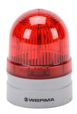
WERMA EvoSIGNAL Mini TwinLIGHT series LED industrial signal beacon, 62mm, red, permanent or blinking (1 Hz ON for 410ms), IP66, modular mount, 12 VAC/VDC. Requires mounting adapter.
