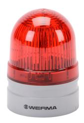
WERMA EvoSIGNAL Mini TwinLIGHT series LED industrial signal beacon, 62mm, red, permanent or blinking (1 Hz ON for 420ms), IP66, modular mount, 115-230 VAC. Requires mounting adapter.
