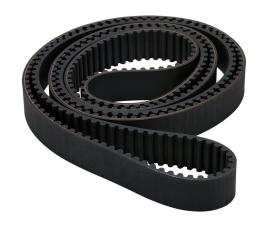
SureMotion timing belt, 8mm 8M pitch, 30mm wide, 325 tooth, 2600mm pitch length (circumference), neoprene, fiberglass reinforced.
