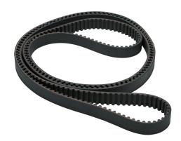
SureMotion timing belt, 8mm 8M pitch, 20mm wide, 325 tooth, 2600mm pitch length (circumference), neoprene, fiberglass reinforced.
