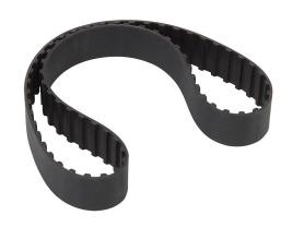
SureMotion timing belt, 3/8in L pitch, 1in wide, 68 tooth, 25.5in pitch length (circumference), neoprene, fiberglass reinforced.
