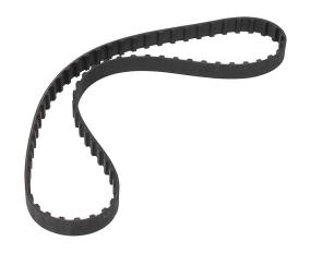
SureMotion timing belt, 3/8in L pitch, 1/2in wide, 68 tooth, 25.5in pitch length (circumference), neoprene, fiberglass reinforced.
