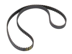
SureMotion timing belt, 1/5in XL pitch, 3/8in wide, 125 tooth, 25in pitch length (circumference), neoprene, fiberglass reinforced.
