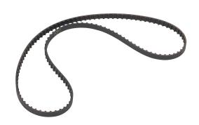
SureMotion timing belt, 1/5in XL pitch, 1/4in wide, 125 tooth, 25in pitch length (circumference), neoprene, fiberglass reinforced.
