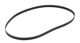
SureMotion timing belt, 0.08in MXL pitch, 1/4in wide, 250 tooth, 20in pitch length (circumference), polyurethane, polyester reinforced. Package of 3.
