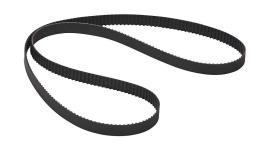
SureMotion timing belt, 0.08in MXL pitch, 1/4in wide, 250 tooth, 20in pitch length (circumference), neoprene, fiberglass reinforced. Package of 3.
