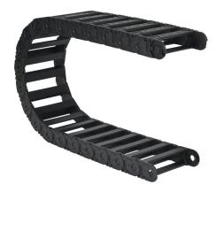
igus 2500 cable drag chain, 0.98in inside height, 4.06in inside width, 4.92in bend radius, outside opening, 1.81in pitch, 3.2ft/1m length, black. Requires 2100-34PZB or 2100-12PZB brackets for mounting.
