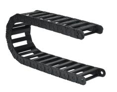
igus 2500 cable drag chain, 0.98in inside height, 4.06in inside width, 3.94in bend radius, outside opening, 1.81in pitch, 3.2ft/1m length, black. Requires 2100-34PZB or 2100-12PZB brackets for mounting.
