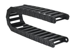
igus 2500 cable drag chain, 0.98in inside height, 4.06in inside width, 2.95in bend radius, outside opening, 1.81in pitch, 3.2ft/1m length, black. Requires 2100-34PZB or 2100-12PZB brackets for mounting.
