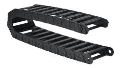
igus 2500 cable drag chain, 0.98in inside height, 4.06in inside width, 2.16in bend radius, outside opening, 1.81in pitch, 3.2ft/1m length, black. Requires 2100-34PZB or 2100-12PZB brackets for mounting.
