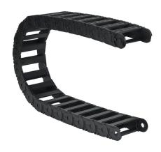
igus 2500 cable drag chain, 0.98in inside height, 3.03in inside width, 4.92in bend radius, outside opening, 1.81in pitch, 3.2ft/1m length, black. Requires 2070-34PZB or 2070-12PZB brackets for mounting.
