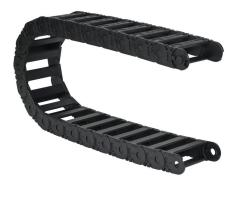
igus 2500 cable drag chain, 0.98in inside height, 3.03in inside width, 3.94in bend radius, outside opening, 1.81in pitch, 3.2ft/1m length, black. Requires 2070-34PZB or 2070-12PZB brackets for mounting.
